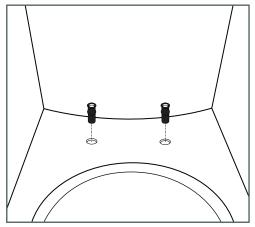
Insert threaded rubber piece into holes on top of toilet.
