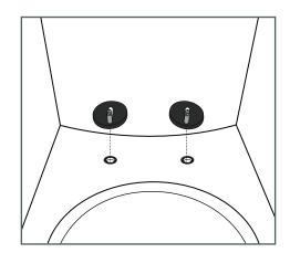
Place seat hardware over where you inserted the threaded rubber pieces.
